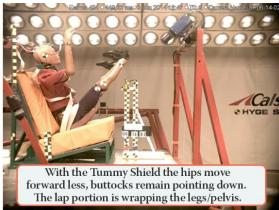
While doing crash testing using an instrumented crash test dummy (Hybrid III 5% female), we compared the dynamics of using only a seat belt with a seat belt and the Tummy Shield. I was surprised to see how deeply the seat cushion was compressed by the test dummy in both scenarios. The video footage shows a noticeable difference in the extent of submarining when using only the
